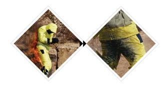
When exposed to heat & flame, the fabric forms a self-extinguishing char that protects the user.
