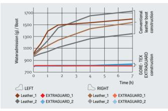
Compared with conventional boots, GORE-TEX EXTRAGUARD boots have very low water absorption, confirmed by the water bucket test.
