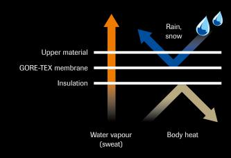
If insulation gets wet with sweat or from water it will lose its insulating properties. Damp or wet insulation will conduct body heat to the outside as much as 6 times faster than when it is dry. It will also feel cold and uncomfortable.
