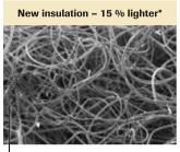
Fewer, lightweight hollow fibres, low fibre density
