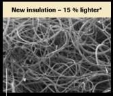
Fewer, lightweight hollow fibres, low fibre density
